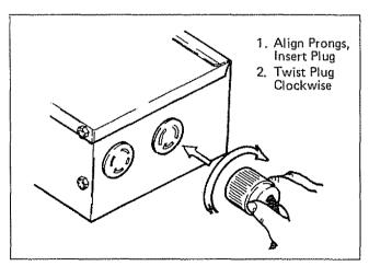
To plug the connector plug into the outlet, line up prongs and insert plug. Then twist plug clockwise to lock.
